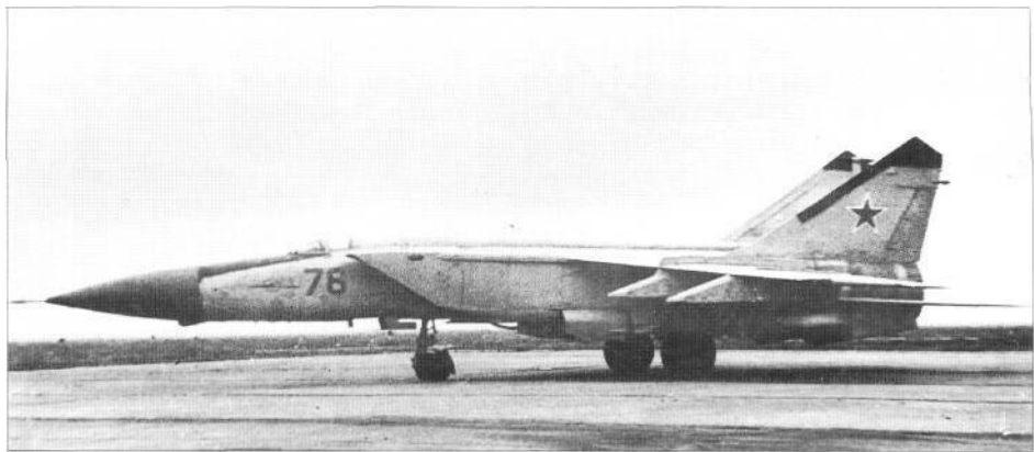
MiG-25P testing the 'Parol IFF system - the small 'bump' at the base of the radome.
